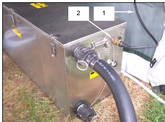
Figure 21. Grease Separator Power Cable Installation.
