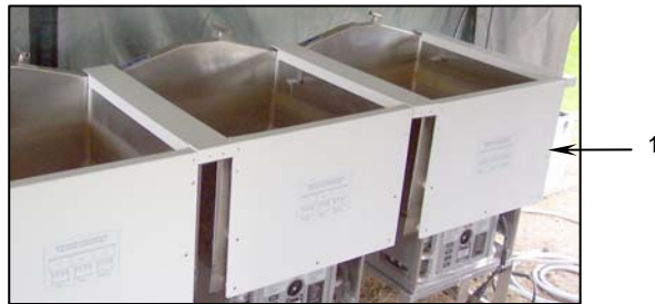
Figure 28. Sink Heat Shield Installation.
